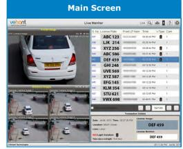
Main Screen displays the live transactional data from connected traffic crossings, including the number plate of the vehicles, location, time and time since red light.
