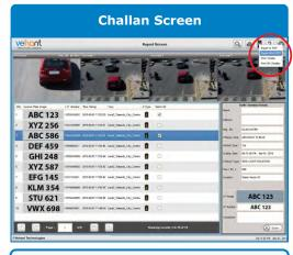
Challan Screen displays the list of red light violating vehicles as per user-defined criteria with details including vehicle number plate, location and time stamp. The operator uses the information to validate and print the challan.
